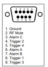
Figure 8.1: Alarms and Triggers Port
