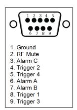
Figure 7.2: Alarms and Triggers Port
