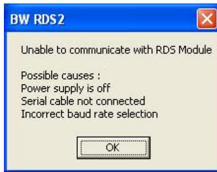
Figure 2.4 BW RDS2 Software Failed Communications sub window.
